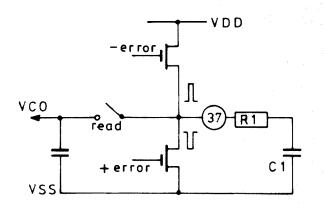
Error between VCO and VCM frequency ratio is integrated in R1 C1, and read out to correct VCO. RC too small causes frequency instability, RC too large causes slow shift to next tone.
