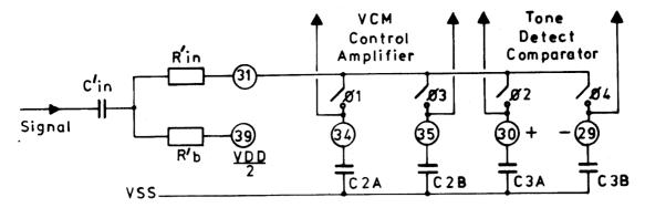
Components: C' in = 0.01 MFD 10%, R' in = 330 K $\Omega$  10%, R'b = 330K $\Omega$  10%
